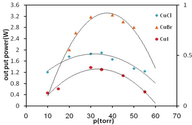
Fig. 5. Laser output power versus neon buffer gas pressure for CuI, CuBr and CuCl as lasants. The left axis is related to CuCl and CuBr lasers and the right one is related to CuI laser.
