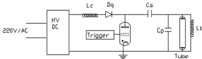
Fig. 2. Schematic layout of standard circuit of CuI laser:
