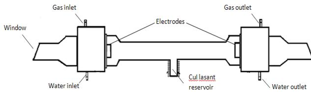
Fig.1. Schematic layout of CuI laser.
