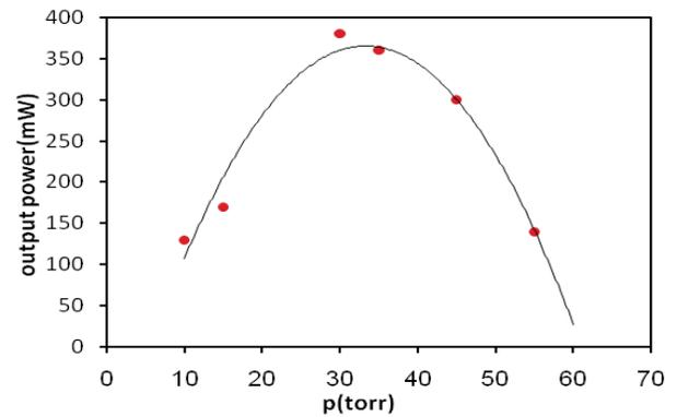
Fig. 3. Average laser output power versus buffer gas pressure.
