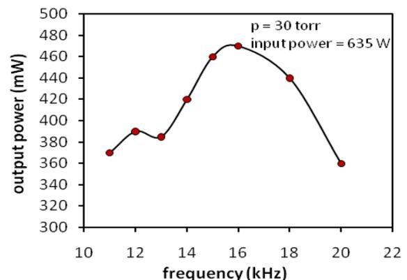
Fig. 4. Laser output power versus frequency.
