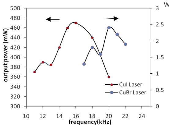
Fig. 6. Laser output power versus frequency for CuI and CuBr as lasants.
