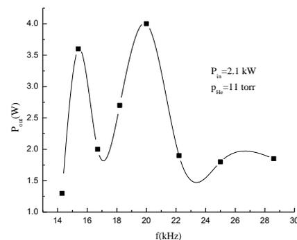
**Fig. 5.** Variation of P<sub>out</sub> versus frequency
