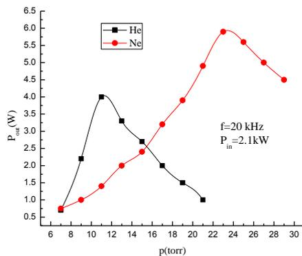
**Fig. 6.** Variation of CBL output power versus He and Ne buffer gas pressure
