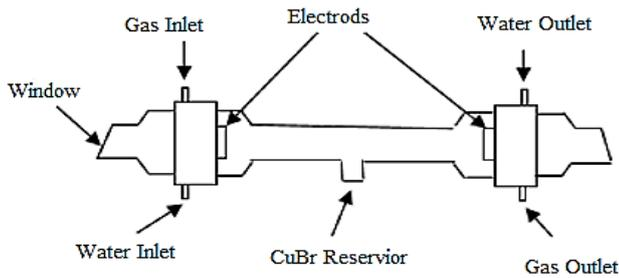
**Fig. 1.** Schematic layout of CuBr laser.
