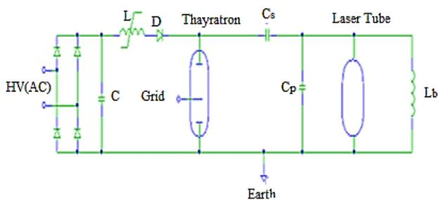
**Fig. 2.** Schematic representation of standard circuit of CuBr laser.  $C_p=0.47\text{nF}$ ,  $C_s=1.65\text{nF}$ ,  $L_b=100\mu\text{H}$ ,  $L=150\text{mH}$
