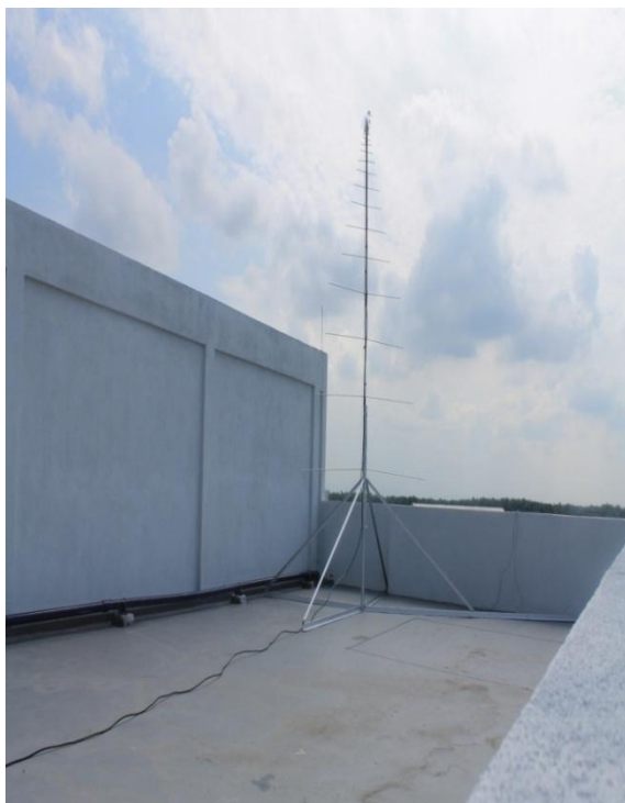
Fig.2 Logarithmic Periodic Dipole Antennas of e-CALLISTO
